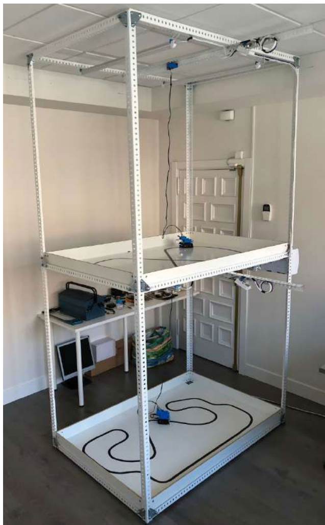
FIGURE 11. LabsLand Arduino Robotics laboratory deployed at LabsLand, in Bilbao. The structure provides two separate experimentation instances.
