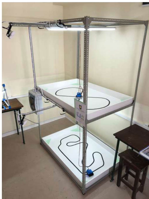
FIGURE 19. LabsLand Arduino Robot Laboratory deployed at the University of Fort Hare, in South Africa. A single structure provides two different experimentation instances.
