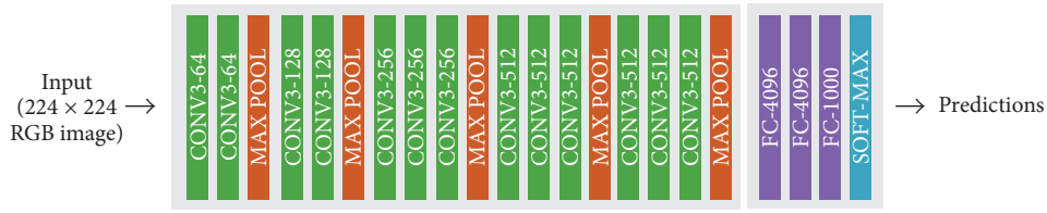
FIGURE 3: VGG-16 architecture: convolutional layers in green, max pooling layers in orange, and fully connected layers in purple. We followed the same notation of the original paper.
