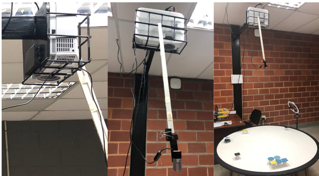
Figure 7. Sandbox table with markers and details of the camera and projector.
