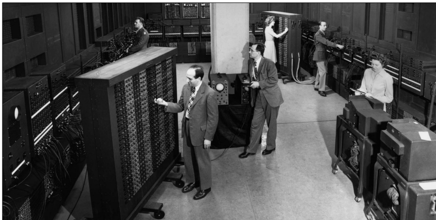
Figure 2.2: J. Presper Eckert and J.W. Mauchly working on the ENIAC, at the University of Pennsylvania in January, 1946. The Portable Function Table (featured in the foreground) contained a series of switches that allowed the operators to modify the functioning of the machine. The punch card reader and writer (bottom-right corner) allowed the data input/output operations.
