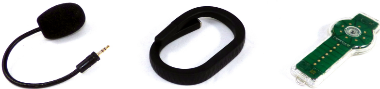
Figure 2.23: Common microphones (left) can be used to register human speech. However, to detect bioelectric input, it is often necessary to employ wearable devices (center) with special sensors in direct contact with the users’ skin. Other external devices (right) can also be fitted with additional sensors to provide complementary control mechanisms.
