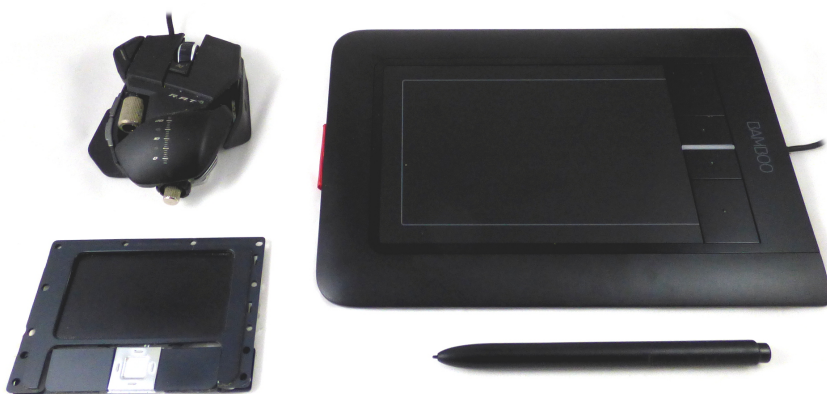
Figure 2.19: Different kinds of 2D pointing devices: a mouse with advanced functions (top left), a touchpad common in laptop computers (bottom left) and a graphics tablet that can be used with a special stylus or as a multi-touch surface (right).
