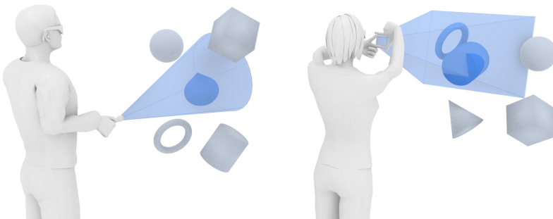
Figure 2.11: Either using a 3D mouse or by tracking the hands of the user, it is possible to create advanced interaction mechanisms that allow the selection of the interactive elements in a SUI.
