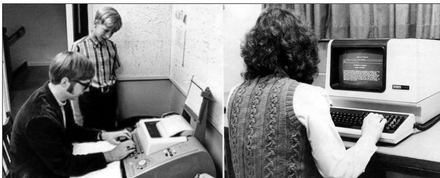
Figure 2.4: An ASR-33 teletype modified to interact with a time-sharing computer system (left) and a DEC VT100 (right), one of the first –dumb– terminals that supported ANSI escape codes (useful for text-based menu navigation).
