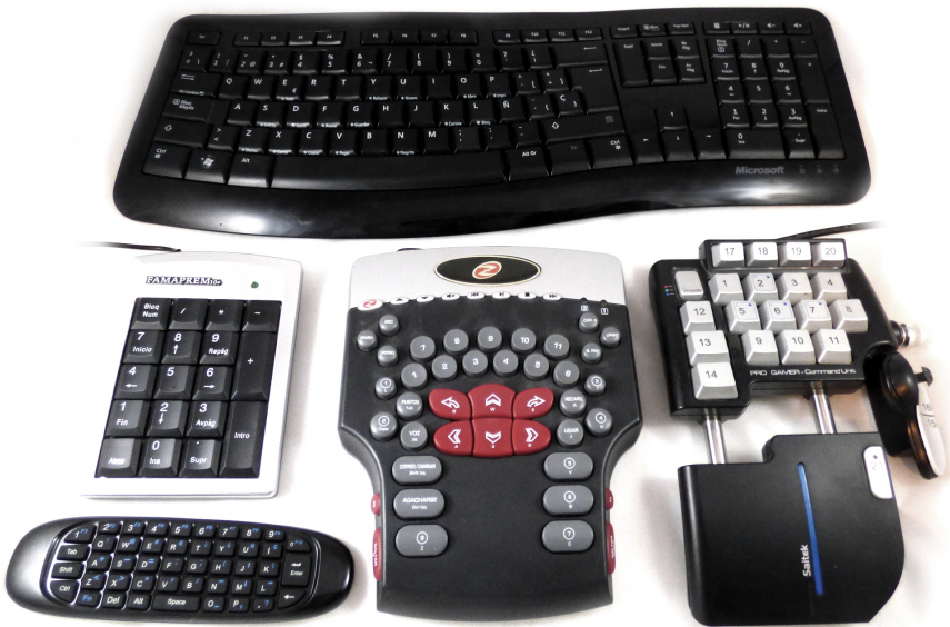
Figure 2.18: Different keyboard types (for specific tasks): general-purpose (top), numeric input (left), –portable– alphanumeric input (bottom left) three-dimensional navigation (bottom center) and system control (bottom right).
