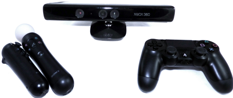
Figure 2.9: With the introduction of Kinect (top), Microsoft experimented to create more intuitive and immersive user experiences by tracking the body of the users. Meanwhile, its rival Sony tried to emulate the success of other platforms by integrating motion-sensing capabilities and, later, touchpads into their game controllers.
