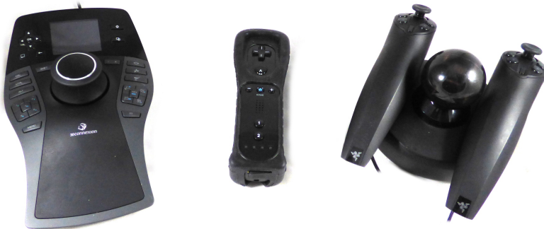
Figure 2.20: On top of providing six DoF, current 3D mice (left) include additional controls to facilitate navigation and system control tasks. Meanwhile, the widespread acceptance of the Wiimote (center) between researchers, encouraged manufacturers to develop their own 3D pointing devices (right).
