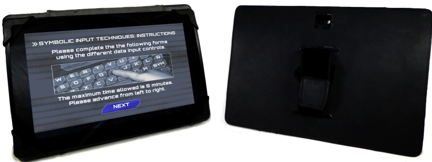
Figure 4.11: The final version of the experimental equipment consisted on a Nexus 10 tablet with a custom-made handler. Please note that the back side of the handler included an adjustable Velcro buckle and a hole for the camera.
