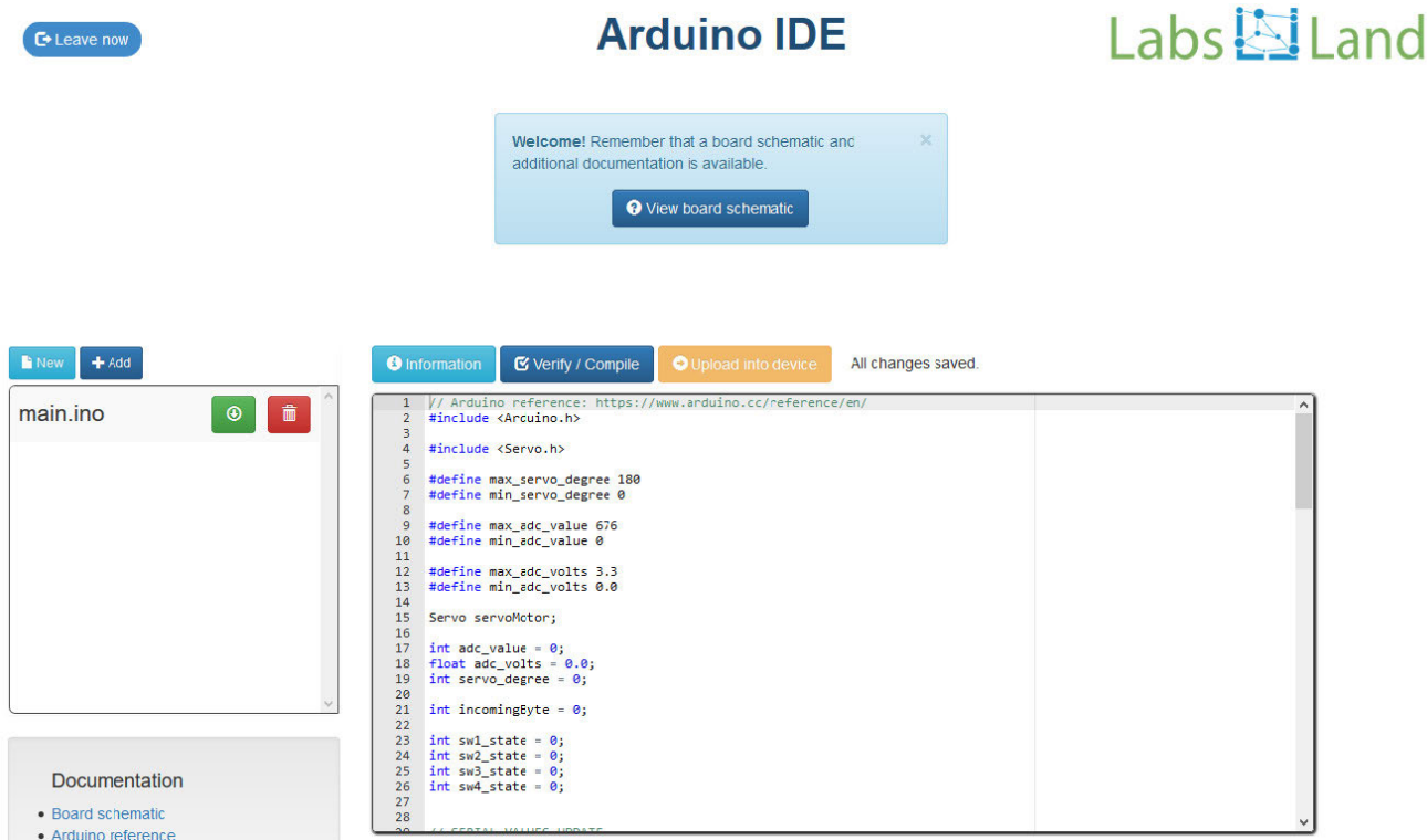
FIGURE 6. Web-based integrated IDE for the ArduinoRL remote laboratory.
