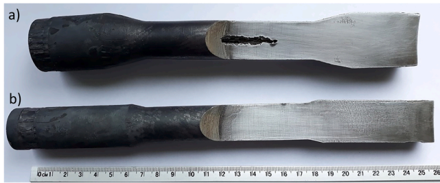
Fig. 7. Samples rolled in the experiments: a) sample rolled at \delta = 1.5 ; b) sample rolled at \delta = 1.18 .
