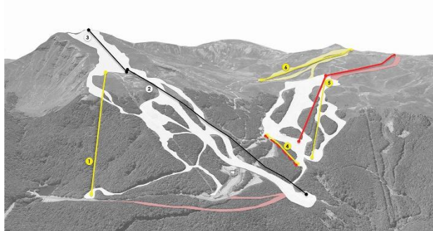
Figure 3. Scenario 3: Expansion and substitution of the existing chairlift
