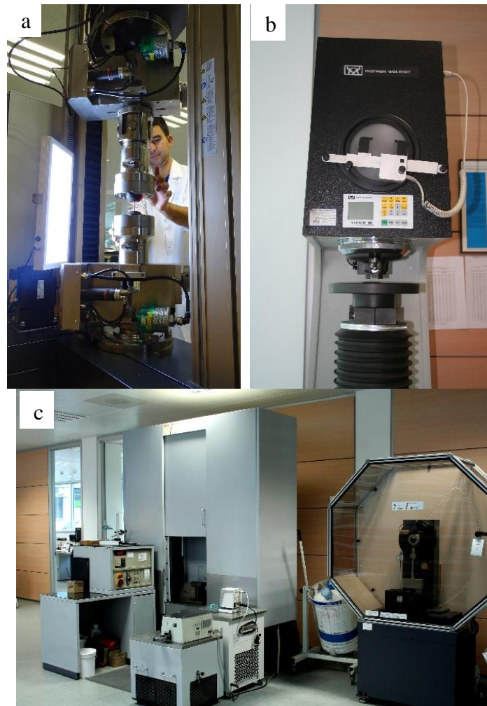
Figure 42. Image of a) Tensile test machine, b) Brinell hardness measurement, c) Charpy test machine.
