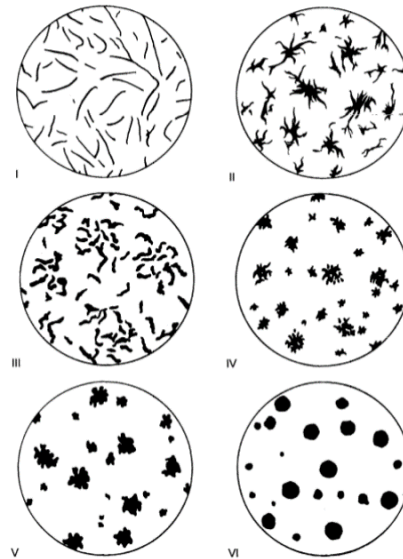
Figure 4. Main graphite shapes in cast iron alloys. Standard ISO 945-1 16 .
