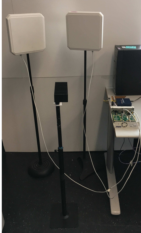
Figure 5.1: The physical RFID system used in the experimental validation. The picture shows an Ettus Research N210 Software Defined Radio, a PC that controls the SDR, a switch to connect the SDR to the PC, two circularly polarized antennas. Alien-9640 tags are attached to foam panels, which are inserted into the black racks.
