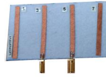
Figure 7: Implementation of the open circuit terminated 50\Omega \lambda/2 microstrip transmission lines over PCPTF/Felt.
