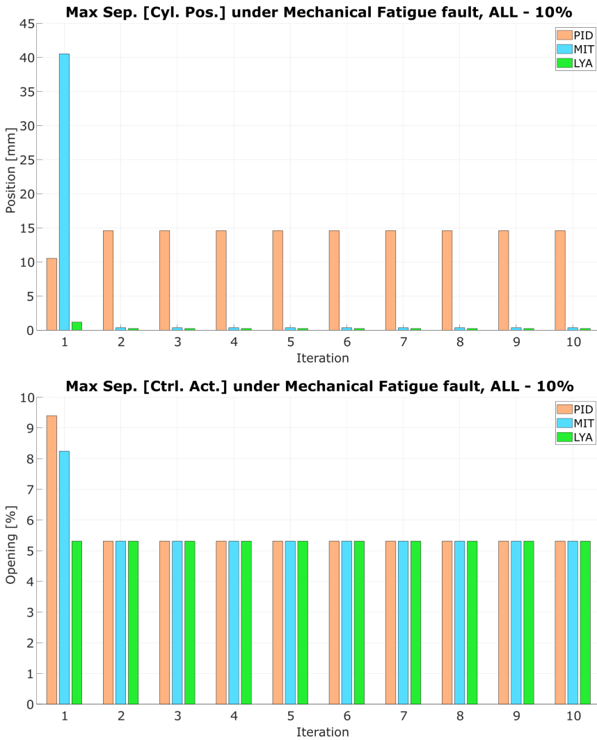
Figure 4.26: Maximum separation between real system and model in a Mechanical Fatigue fault for all the controllers, performance against a 10% fault.
