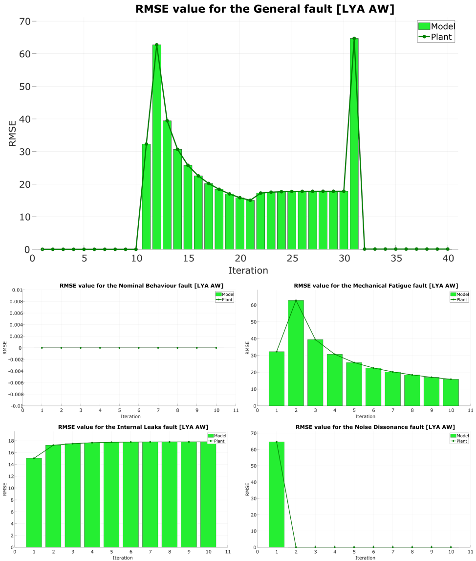
Figure 4.106: Root Mean Square Error between model and plant for several faults with varying loads, performance against a 90% fault.
