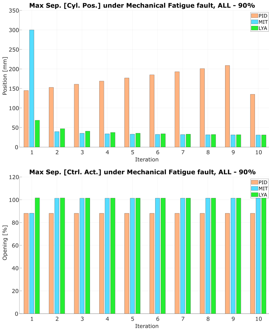
Figure 4.28: Maximum separation between real system and model in a Mechanical Fatigue fault for all the controllers, performance against a 90% fault.
