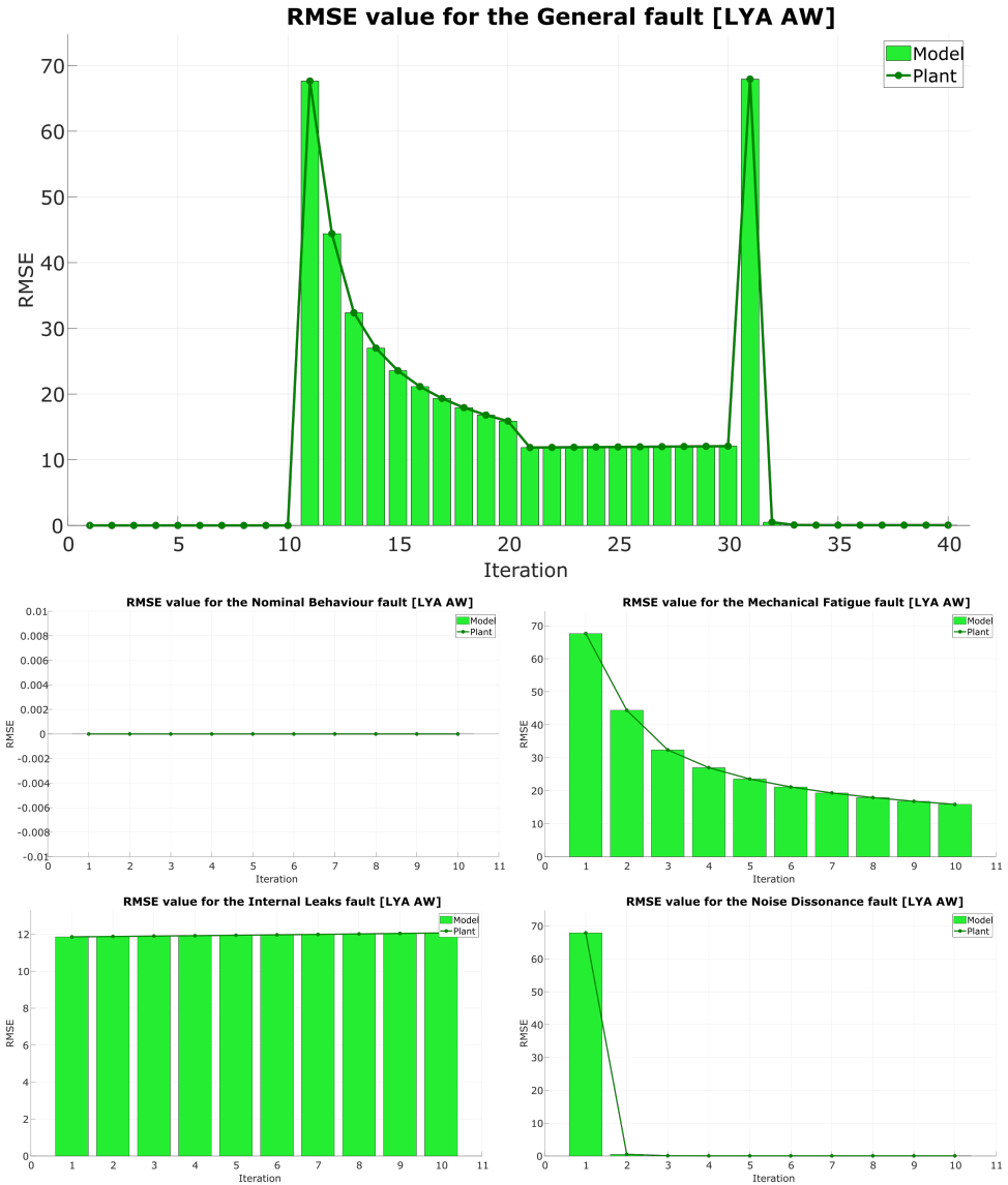
Figure 4.104: Root Mean Square Error between model and plant for several faults, performance against a 90% fault.
