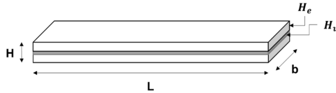
Figure 4. Configuration of the magnetorheological elastomer (MRE)-sandwich structure.
