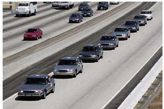
Fig. 3. PATH Program Eight-Car Fully-Automated Platoon Demonstration [20].
