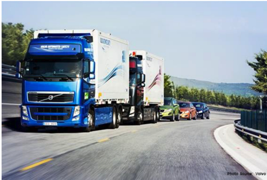
Fig. 8. SARTRE project, two trucks and three passenger cars following leading trucks [27].
