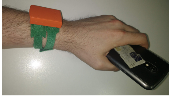
Figure 3.2: Equivalence between handheld and wrist-worn inertial sensors: hardware installation
