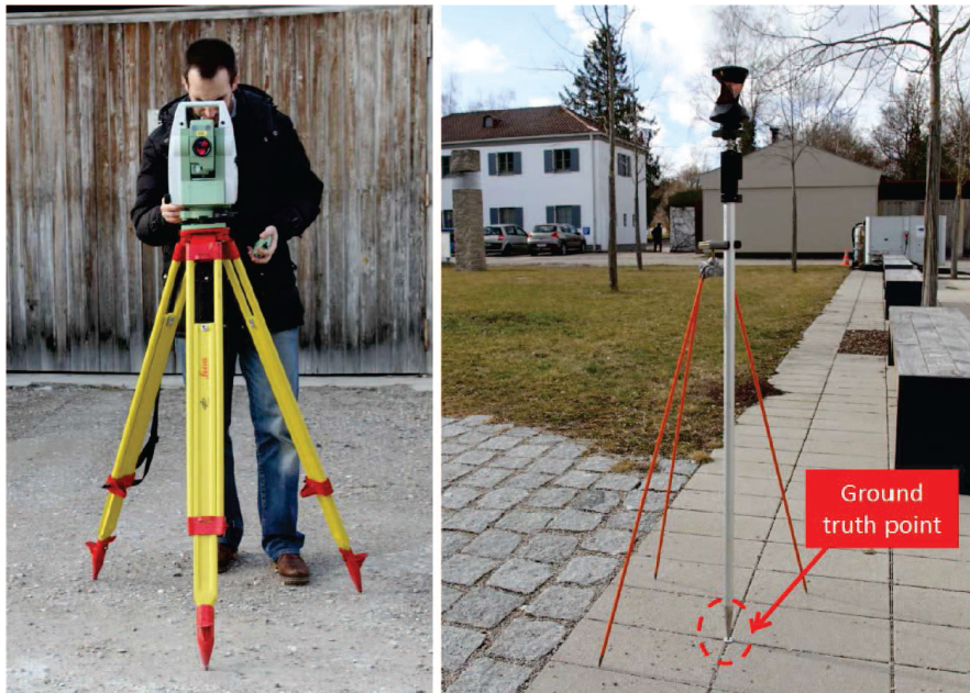
(b) (Left) Leica tachymeter. (Right) 360° prism located on top of a GTP.
