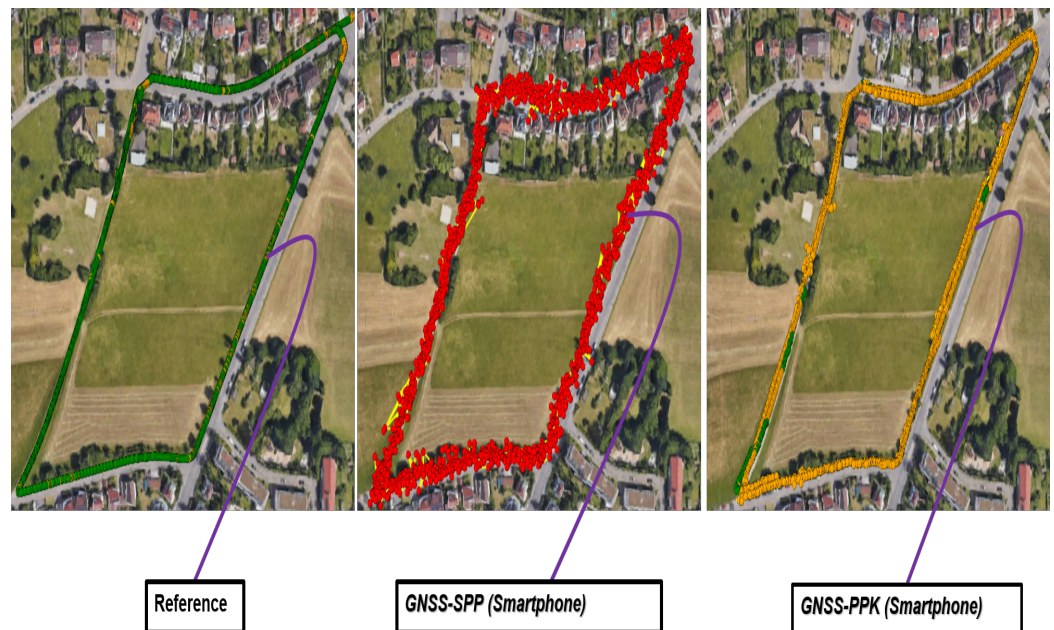
Figure 5. Difference between the ground truth, SPP-GNSS, and PPK-GNSS data.
