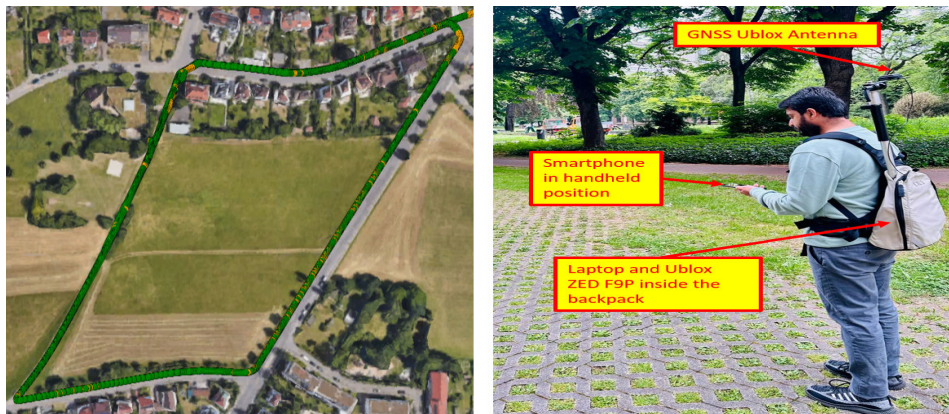
FIGURE 7. Experimental setup and data collection for GNSS error analysis: ground truth and configuration overview.
