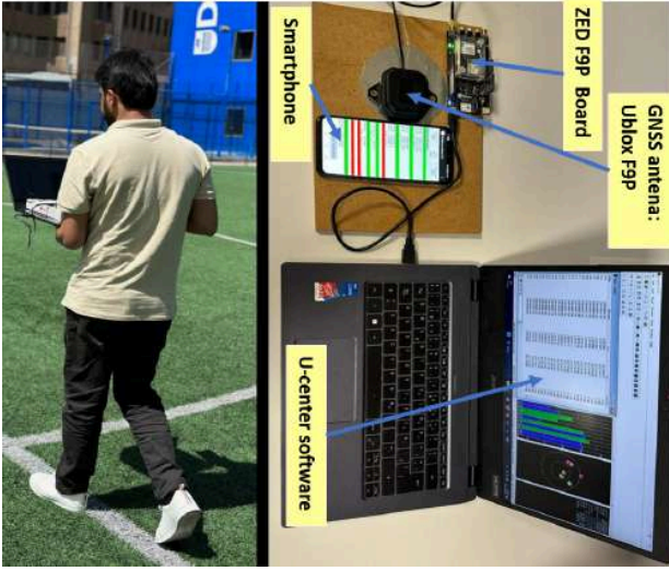
Fig. 5. Data collection and experimental setup.
