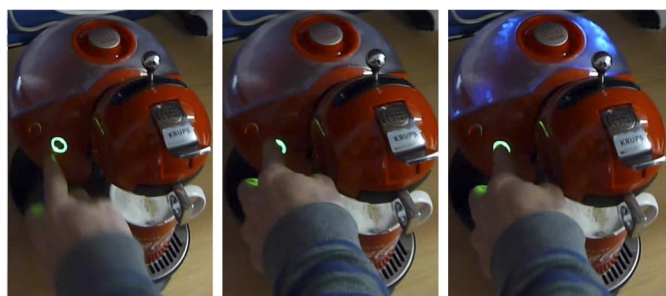
Fig. 3. The persuasive coffee makers provided just-in-time visual cues to help users in energy efficiency decision-making. On the first image, a user approaches its finger to switch off the device. In the second and third pictures, the augmented appliance detects the motion close to the button and informs the user to not switch it off by activating a built-in visual alert. As can be observed in the first picture of Fig. 2, the subtle message to prevent the operation of the appliance is “Please, leave me on”.
