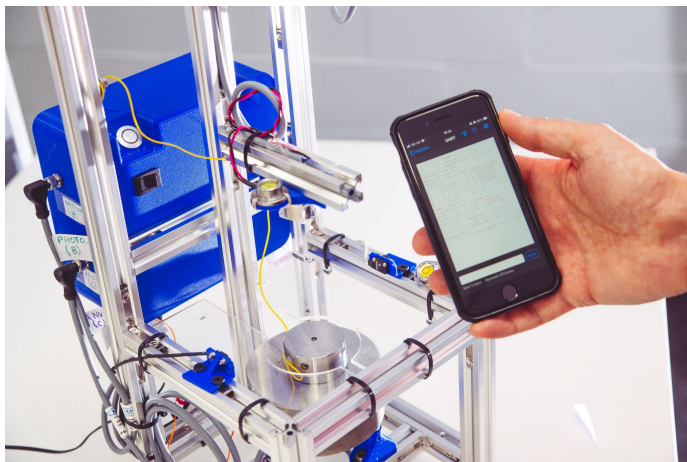
Figure 4.16: The device communicates through BLE UART terminal emulation. Any smartphone can connect to the device by installing an open-source app.
