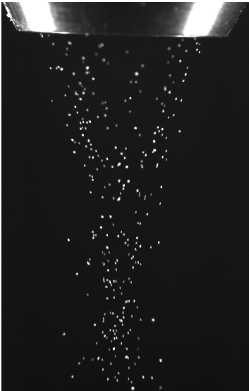
(c) Side illumination result: 3530 fps, 3× gain, 90 \mu s exposure
