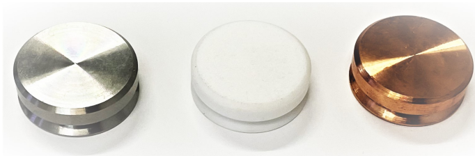
Figure 4.14: Examples of sample stubs as-manufactured, prior to surface polishing. From the left, the materials are AISI 316L steel, PTFE, unalloyed copper (99.9%).
