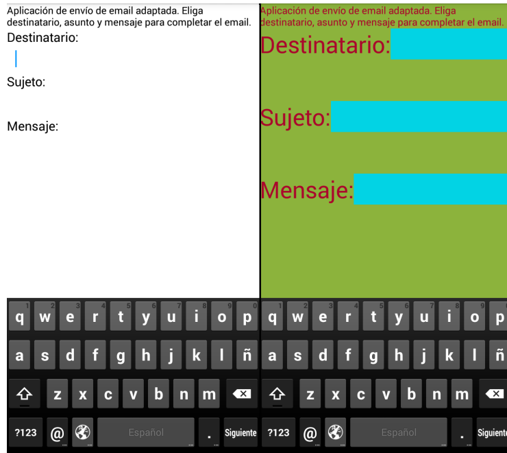
Figure 4.9: User interface adaptation performed by the Adaptation Engine. On the left, a default activity with no adaptation. On the right, the same activity after the adaptation process. As is shown, the colours sets and sizes of each component of the adapted user interface are different from the non adapted one.
