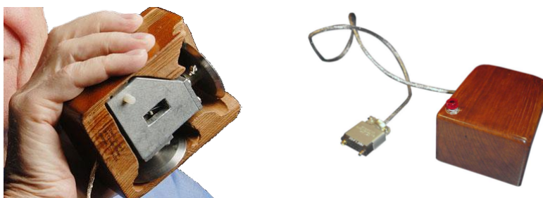
Figure 1.1: First computer mouse by Douglas Engelbart, formed by two wheels representing the two axis on the display, and a single button.
