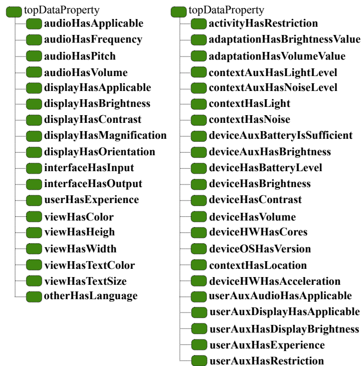
Figure 3.7: AdaptUI datatype properties, not considering other ontologies. The left group of properties are those related to the UserCharacteristics class.
