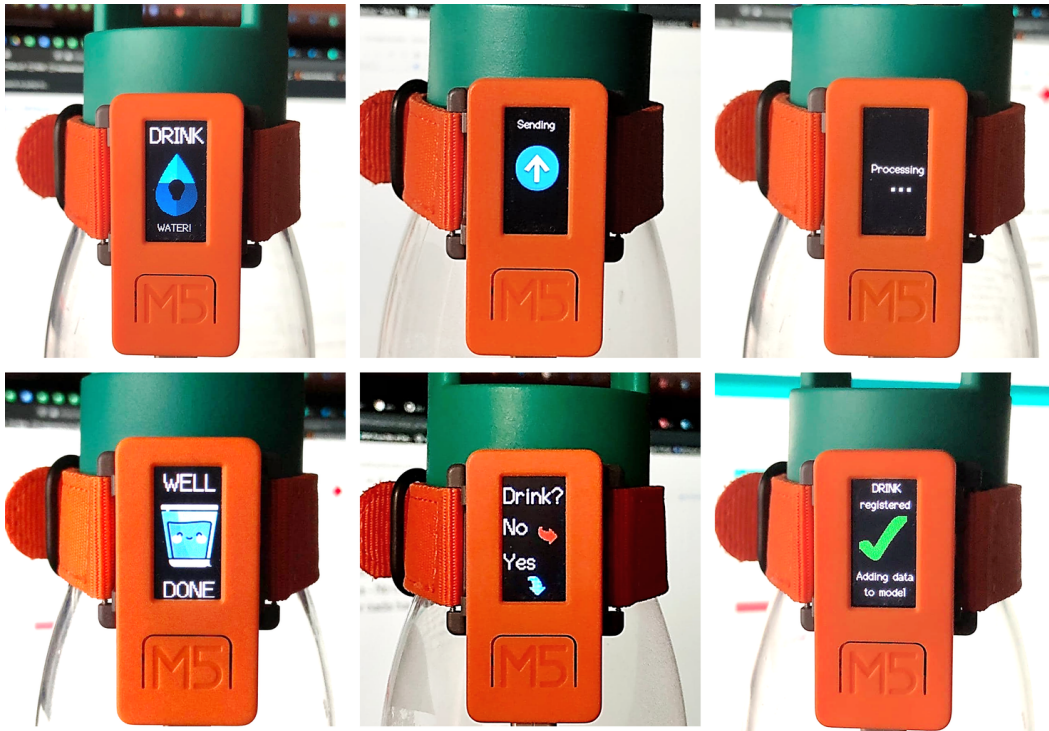
Figure 6.5: A sample of the messages that are prompted through the device's display to interact with the user.
