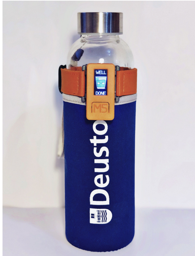
Figure 4.2: The IoT sensor used to collect motion signals placed on one example of the employed liquid containers.
