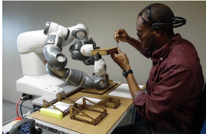
Figure 5. Real experimentation using EEG for an assembly task [33].
