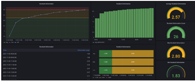
Fig. 13. Grafana dashboard presenting rocks deformation.
