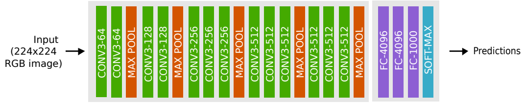
Figure 3.3: Architecture of the VGG-16 network. Green blocks are convolutional layers, orange blocks are max pooling layers, purple blocks are Fully-Connected layers, and the blue block is a softmax activation. From the work of Nunez-Marcos et al. (2017).
