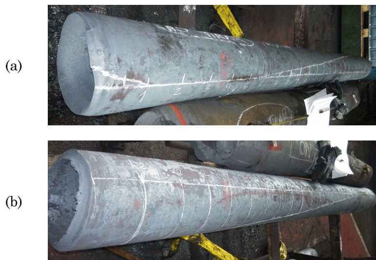
Figure 2. Longitudinal tube torsion: (a) view of the head of the tube and (b) view of the tail of the tube.
