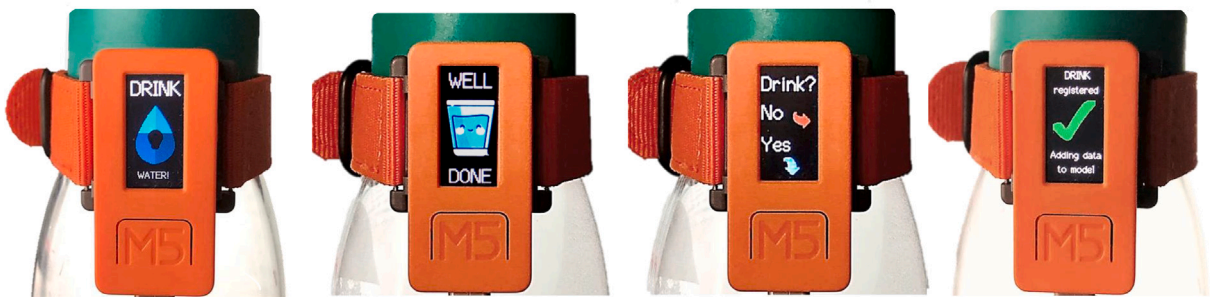
Fig. 2. A sample of the messages that can be prompted to a user when detecting a hydration activity through the device's display. As can be seen, in some cases, the drinking gesture is automatically detected, while, in case of uncertainty, the user must provide validation feedback to confirm the performed gesture.
