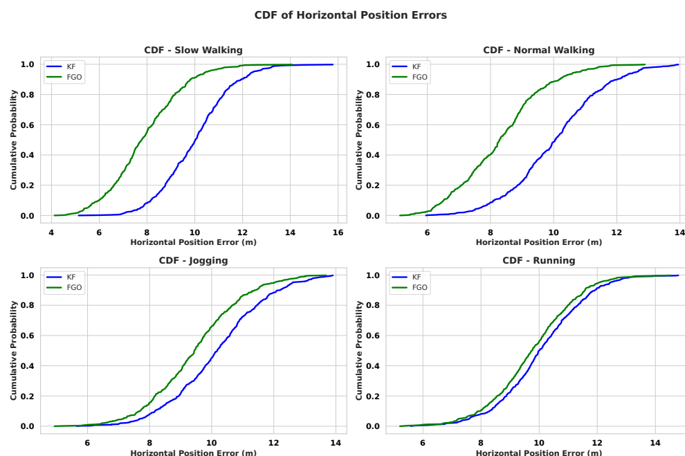
Figure 7. CDF of horizontal position errors (HPEs) aggregated over all pedestrians for different motion types: slow walking; normal walking; jogging; running. FGO consistently achieves higher cumulative probabilities at low error thresholds compared with KF, despite inter-subject variability.
