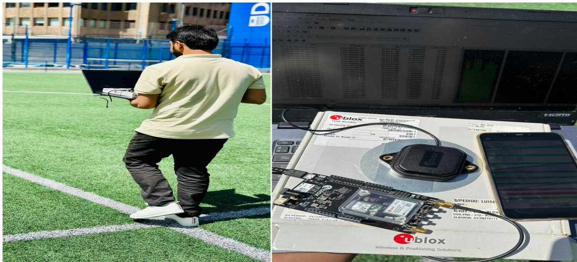
Figure 3. Data collection and experimental setup: (left) pedestrian carrying the smartphone during outdoor data collection; (right) ground-truth GNSS setup consisting of the Ublox ANN-MB-00-00 antenna connected to the ZED-F9P processing board.
