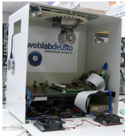
Figure 8. An instance of the WebLab-FPGA hardware, shared by the traditional WebLab-FPGA and the Hybrid one.
