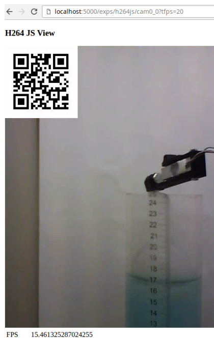
Figure 2.6: Interactive live-stream with an embedded QR timestamp to measure the true capture-render delay.
