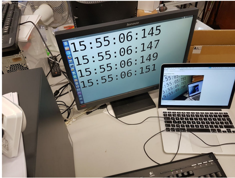
Fig. 5 Picture measuring the capture-render delay
