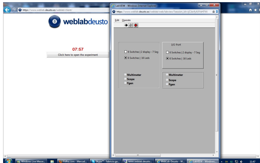
Figure 3.11: LabVIEW Remote Panels integrated in WebLab-Deusto. Configuration screen.
