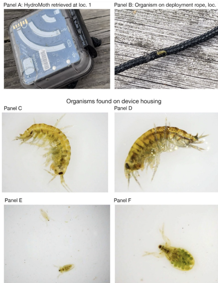
Figure 3 Documentation of organisms that came to inhabit and co-opt the HydroMoth field recording device in the waters of the Charles River, Boston, MA (Gonzalez Quintero & Offenhuber, this track).
