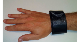
Fig. 7. Designed textile coil embedded in a leather bracelet.
